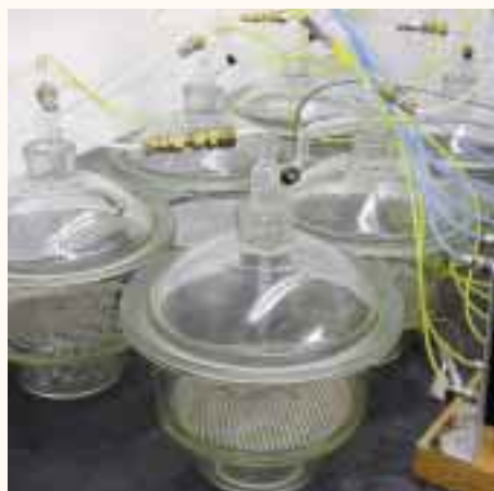
Laboratory tests are used to determine effective dosage rates for phosphine against the major stored grain insect pests.
